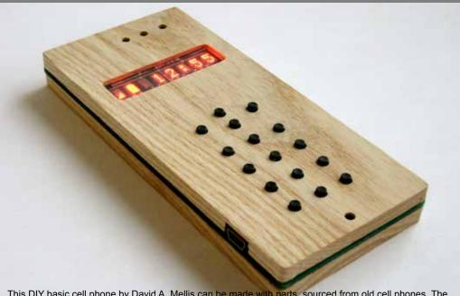
This DIY basic cell phone by David A. Mellis can be made with parts, sourced from old cell phones. The circuit board can be particularly useful in this regard, as well as the display.
